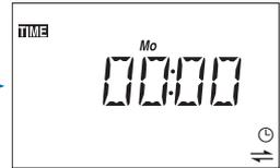
**Step 2:** Use the Item button to advance to the next item. If your installer has selected Daylight Savings Time the date is displayed. If the date has not been set, it will flash. If your installer has not selected Daylight Savings Time, the date will not be displayed.
